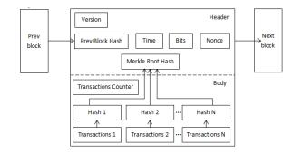
FIGURE 1. Block structure in blockchain system.
