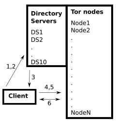
Fig. 1: Current architecture of Tor (simplified).
