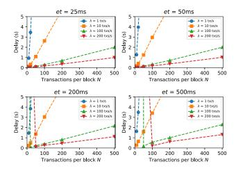
Fig. 4. Transaction delay vs transactions per block with different values of execution time
