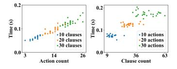
Figure 2: Formal verification performance. The above charts illustrate how the number of actions (left) and clauses (right) affect the time required by Z3 to verify 150 randomly generated agreements. The number of actions and clauses respectively resulted in a correlation of r = 0.97 and r = 0.86 with the time performance of Z3. These results illustrate the more significant impact on prover performance from each action, or free variable, which increases the search space.
